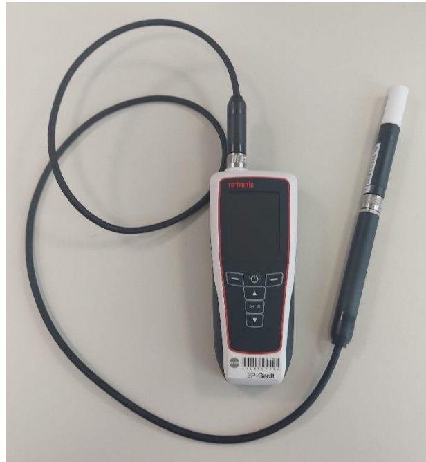
Figure 1: Calibration item: Humidity sensor with measuring device
